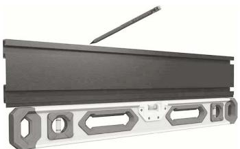
Hold first 24" rail against wall at selected location. Check level, and draw a line along the top of the rail.
