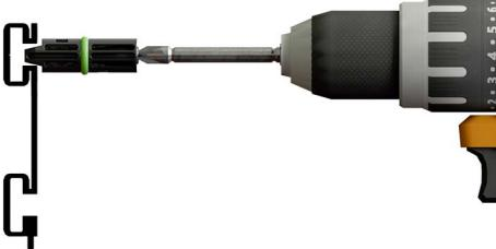
Level the rail and drive screws at each stud location in both the top and the bottom channels of first 24" rail section.
